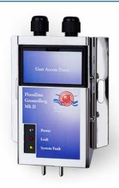
The Floodline Groundhog Mk II is a self-contained, single-zone leak detection system which can be mounted vertically or horizontally. It can be connected to any control/building management system that has the facility to accept volt-free contacts.
