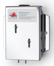
The Floodline Point Sensor is a compact sensor for vertical or horizontal mounting. Water touching its stainless steel probes activates the alarm. Used with the stainless steel Floodline Guard Plate to give heavy duty physical protection and assist fixing and adjustment.
