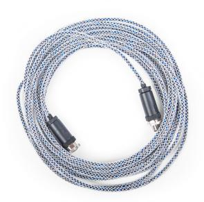
Dedicated to the hybrid leak detection system, the M-line sensor cable detects the presence of water along its entire length. Connected to of the LG24/X control panel identifies a leak on the indicated meter. Wire can be used any number of times (after flooding it is enough dry), is made of a polymeric material with constant properties electric. In the event of damage, the M-line cable can easily be replaced, cleaned and re-installed.
