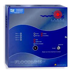
The Multi–Zone Control Panel operates the network of leak detection zones. A zone can be a single point or many metres long and the whole network is continuously monitored for leaks and continuity. Zones are electrically isolated from each other and individually displayed so the system can accept and report any number of simultaneous or consecutive zone alarms – true multiple leak reporting – an alarm in one zone has no affect on the normal monitoring of its neighbours or the rest of the system.
